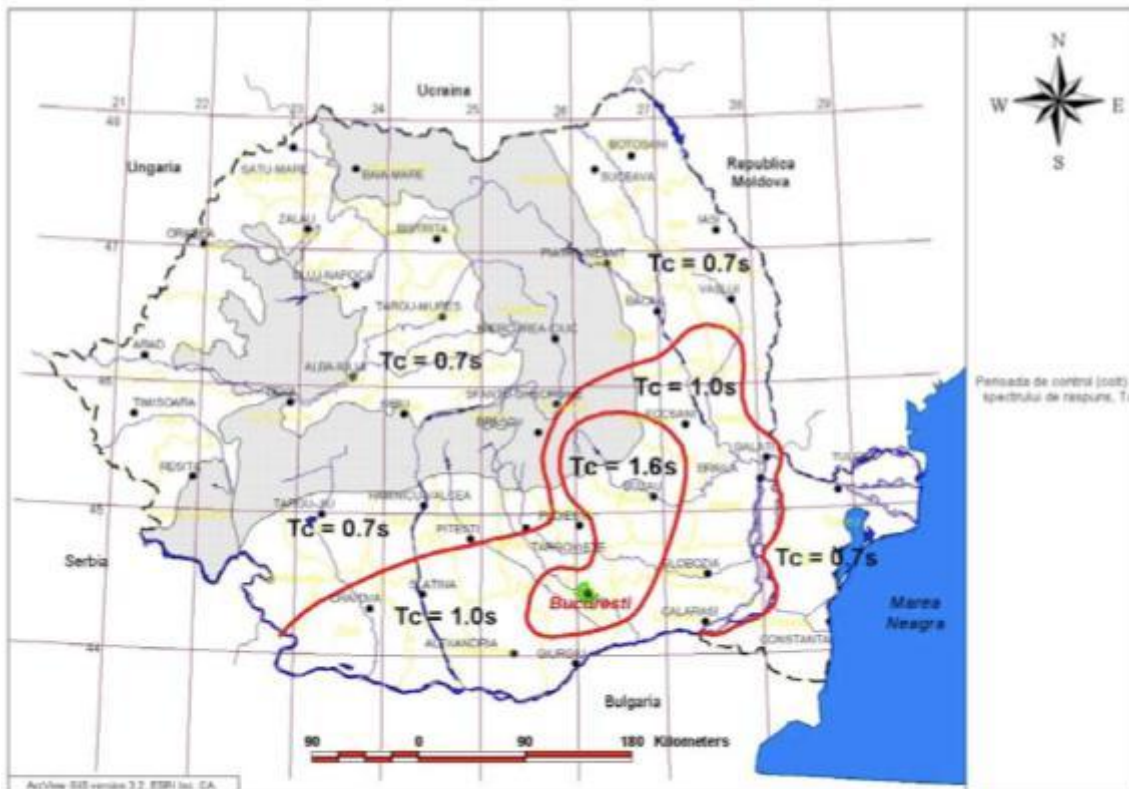
Figure 21: Seismic zoning of Romania in terms of control (corner) periods T_c of the response spectra (P100-1/2006)
